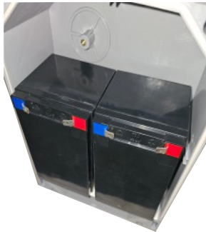
Second battery placed in position
